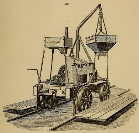
a shape that when half filled with material, and turned round on its axle, the material enclosed is turned over, sideways as well as endways, four times by each single revolution of the mixing vessel. It is fitted with strong top and bottom doors, and is made to revolve on its central axis by means of wheel and pinion gear, and is mounted on a trolly suited to any gauge of rails, or it may have plain wheels for an ordinary road.
